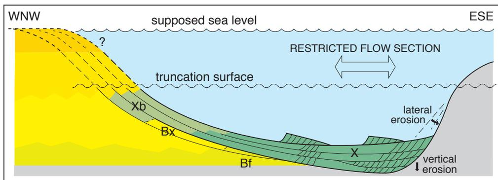
subhorizontal or dip a few percentages to the NNE. The thick cross beds of Archennes seem to be connected with the Bierbeek X facies to form one long body of coarse-grained, thick cross-bedded sand, which hugs the steeper east flank of the Archennes channel (Fig. 2). This body appears to continue to the North.
