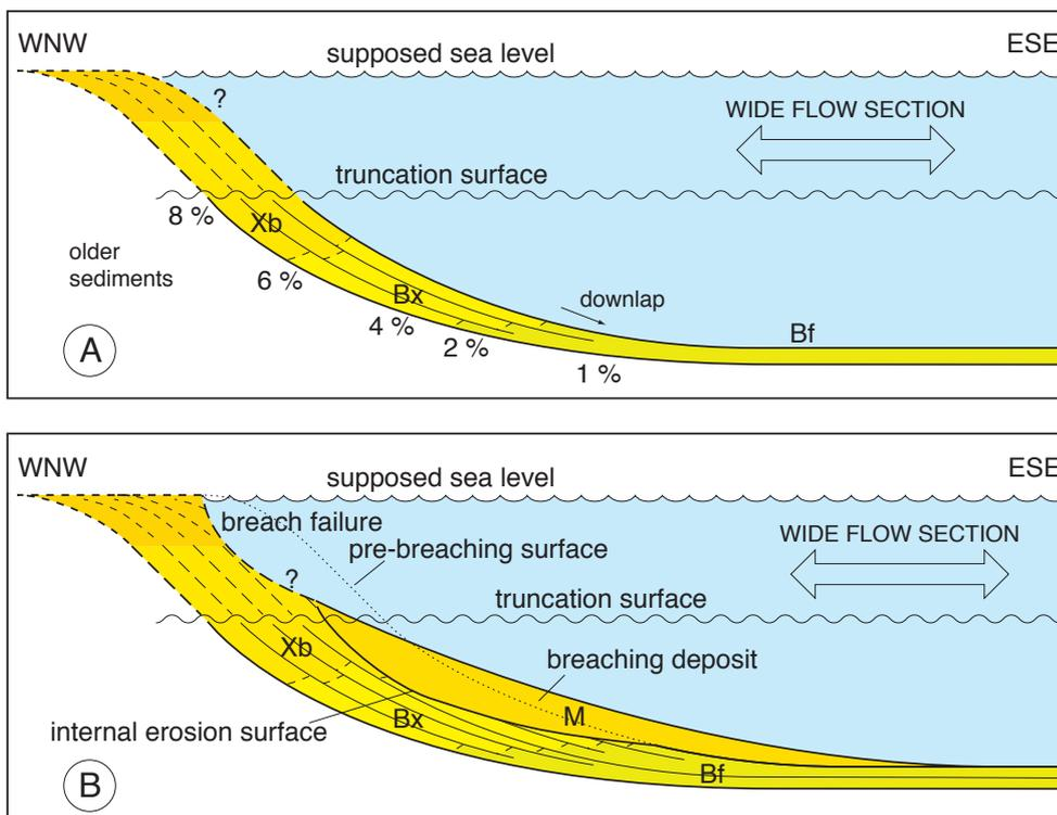
**Figure 9.** Principle of westerly lateral accretion. A : general layout of the lateral accretion arrangement forming a progradational, western shore of the Brussels Basin. Main flow direction is SSW-NNE, perpendicular to the profile. B : Slope apron of facies M partly cut into the westerly lateral accretion arrangement and covering the foot of the shore slope. The truncation surface in A and B is posterior to the deposition of the Brussels Sands.
