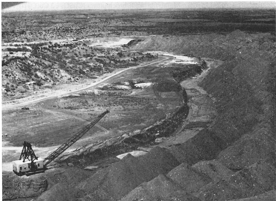
FIG. 6. — Oblique aerial photograph of Eagle-Picher Industries copper-shale strip mine at Creta. Highwall here is 13 m high.
