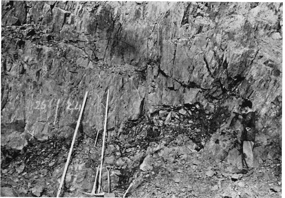
PLATE 3. — Deep glacial shears at 10 m depth in slaty tuffs at Wet Sleddale dam.
