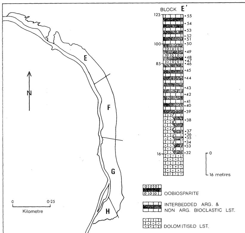
Fig. 2. — Map of the Malahide coastal exposure (after Smyth, 1920) with a vertical section of Block E showing the sampled horizons.
