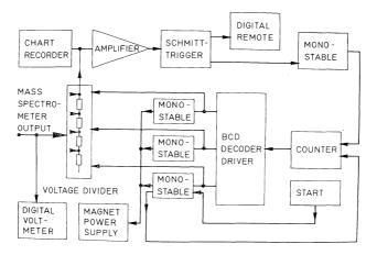
is delayed in a monostable multivibrator circuit. The delay time depends on the type of mass spectrometer. The multivibrator output signal is connected to the BCD counter. At the BCD output, the coded information is stored ,as mass number, voltage range, scan speed and time.
