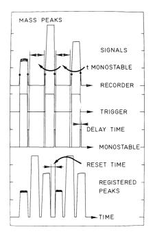
The first peak appears. On a defined voltage level the Schmitt-trigger switches from off to on. At the negative peak edge, the trigger switches off again. This offswitching pulse causes a delay signal from the following one shot. The one shot goes to the logic and it says for example :
