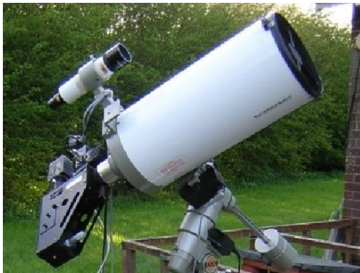
Figure 4: The private Three Hills Observatory of Robin Leadbeater in Cumbria / England consisting of a Vixen 20cm Cassegrain and an off-the-shelf LHIRES III Littrow slit spectrograph
