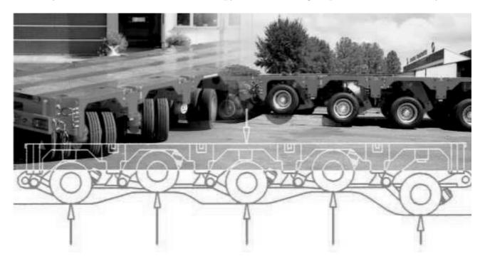
Figure 3: Features of a module transporter.
