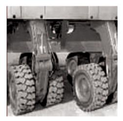
Figure 2: Wheel boogie of module transporter.
