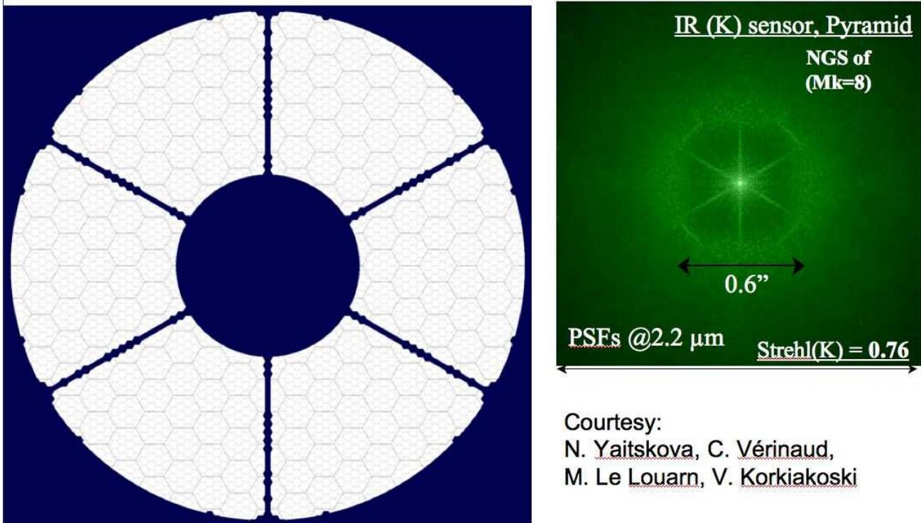
Figure 2: Typical simulated PSF (right) of an adaptive corrected OWL segmented pupil (left). The main PSF structure arise from the so-called *missing segments* (segments behind the mechanical support structure of the secondary mirror, in six-fold symmetry), from the secondary and primary mirror segmentation. The PSF is displayed in logarithmic scale.
