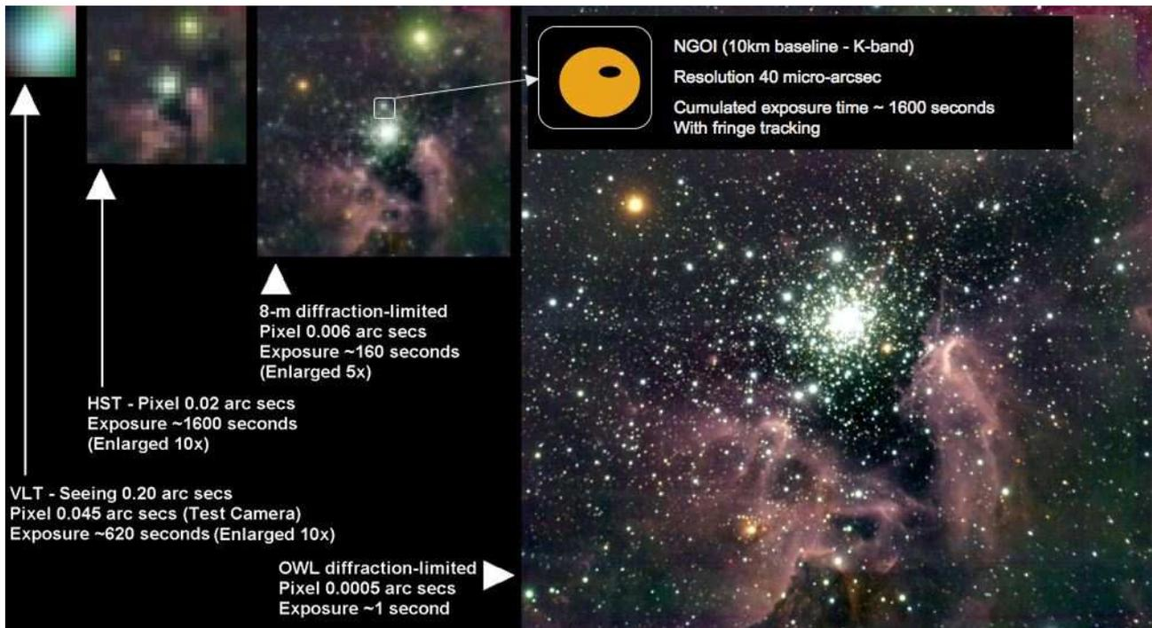
Figure 1: Resolution and sensitivity of different type of telescope: 8-meter-class ground-based seeing-limited telescope, 2-meter-class space telescope, 8-meter-class diffraction limited telescope and 100-meter-class diffraction limited telescope (courtesy ESO OWL team). The resolution and field of view of an NGOI is superimposed as a resolved elongated star with a spot.
