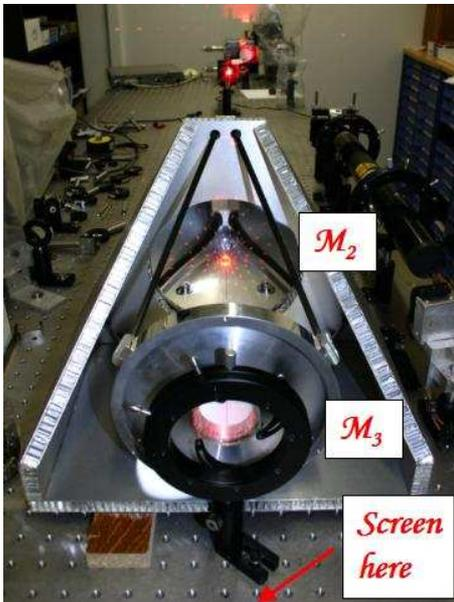
Figure 11: *Hartmann testing of the Mertz corrector in the laboratory. The corrector is back-illuminated by a laser, through a micro-lens array. The spherical aberration, evidenced by the distorted grid pattern of the spots on the mirror  $M_2$ , is correctly corrected if non-distorted in the plane of  $M_1$ .*
