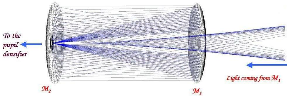
Figure 10: *Beams propagation into the spherical corrector of aberrations drawn with Zeemax (J. Dejonghe).*
