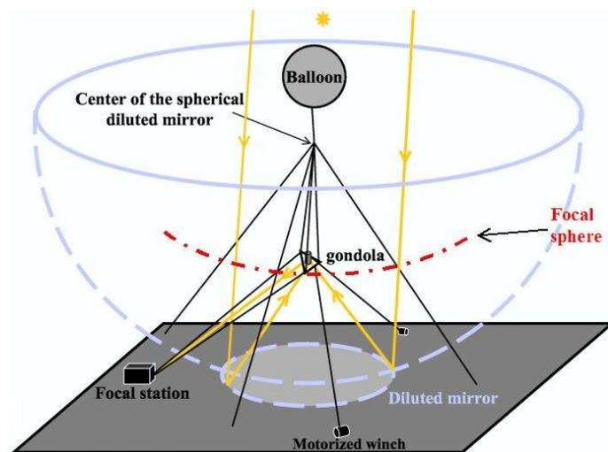
Figure 6: *Optical design of Carlina. The light coming from the star is reflected by the primary mirrors on the gondola at 35 m from ground. The shape of the primary mirrors avoids the use of delay lines because all optical paths are coarsely equalized by the spherical mirror, and finely equalized by the Mertz corrector. The gondola moves along the focal sphere, thanks to the winches, in order to track the star.*
