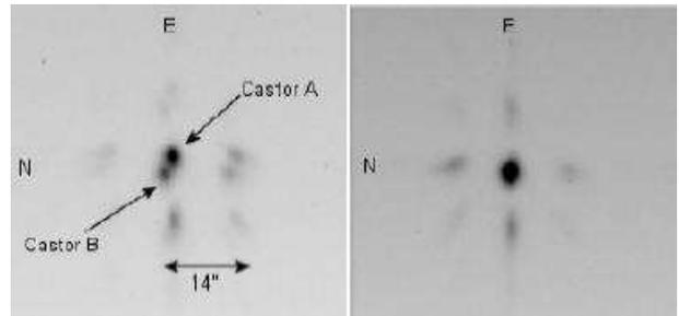
Figure 5: *Image of Castor on the left and Pollux on the right obtained with a  $74 \times 1\text{mm}$  sub-apertures hypertelescope with a 10 cm baseline (Gillet et al, 2003).*
