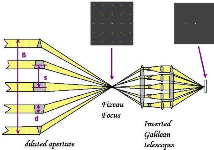
Figure 1: Principle of hypertelescopes. From left to right : the diluted interferometer; at the Fizeau focus, the image consists of a central peak amidst dispersed secondary peaks; the 2<sup>nd</sup> lens collimates the beams; the series of diverging lenses and converging lenses form inverted galilean telescopes which enlarge the beams. The last lens focuses all the beams. The resulting image consists of a very intense peak with weaker secondary peaks (see upper right image).
