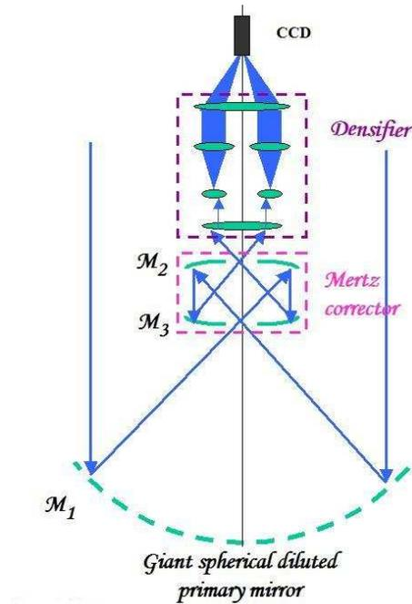
Figure 7: *Optical setup of Carlina*
