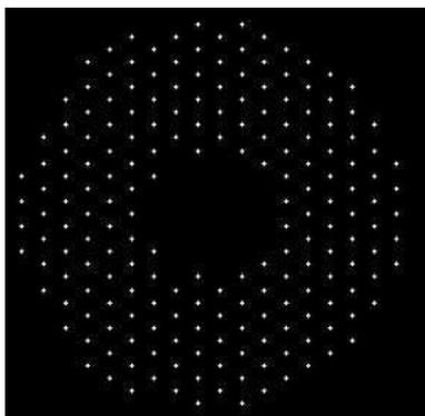
Figure 2: Example of an entrance pupil. The maximum densification factor can reach 4.
