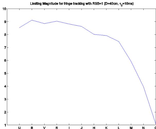
Figure 3: Limiting magnitude for fringe tracking with a signal to noise ration equal to 1, telescope diameter equal to 40 cm and  $\tau_0$  equal to 10 ms. (average conditions at 30 m)
