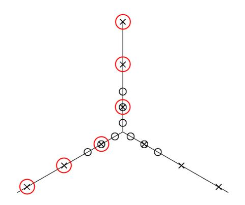
Figure 5: Y-shaped array layout for optical interferometry. Compact and wide configurations (small black circles and crosses) provide different resolutions. Quasi-uniform telescope spacings (large red circles) optimize fringe-tracking efficiency.
