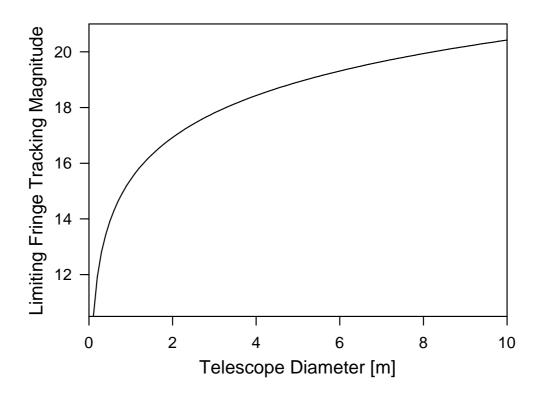
Figure 3: Limiting sensitivity for fringe tracking in the R band as a function of telescope diameter. This estimate is based on an assumed efficiency of 25%, a Greenwood frequency  $f_g = 40$  Hz, and the assumption that 100 detected photons are required per time interval  $1/f_g$  for the fringe tracking servo to work reliably.
