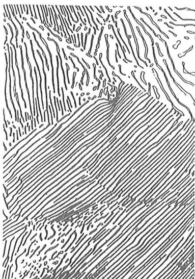
Fig.5. Microstructure of the pearlite in carbon steel used in experiments.
