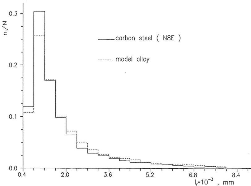
Fig.7. Experimental distribution of random interlamellar spacing. Continuous line – carbon steel; broken line – model alloy.
