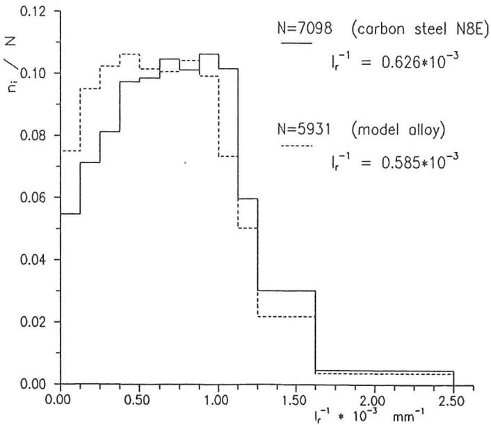
Fig.8. Experimental distribution of random interlamellar spacing inverse. Continuous line – carbon steel; broken line – model alloy.
