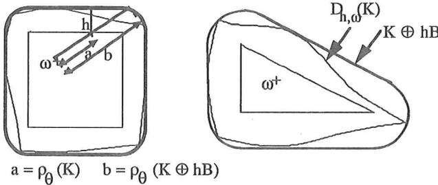
**Figure 3 .** Radial dilation of a square and a triangle, and illustration of (5).
