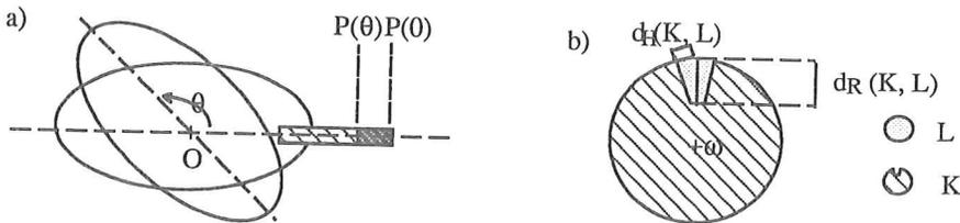
Figure 4 . 4a : movement of a piston given by the rotation of an ellipse.
