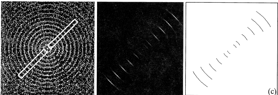
Fig. 3. Illustration of the Fast Fourier Transform algorithm : a) Fourier spectrum and the 45° mask drawn in white ; b) inverse Fourier transform calculated in the 45° mask ; c) the resulting detected continuous portions of circles in a direction close to 135°.
