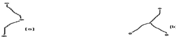
Fig. 2: The labelled points of fibres for a plain fibre (a), and for three endpoints (b).
