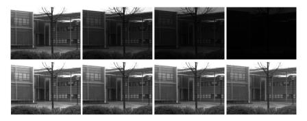
Figure 1. Sequence stabilization. Top line: images under variable exposure times. Bottom line: corresponding images after stabilization
