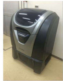
Figure 3. Whole view of the 3D printer. The maximum layer thickness of 3D printing is 15 \mu m. The spatial resolution is 635 \times 400dpi.
