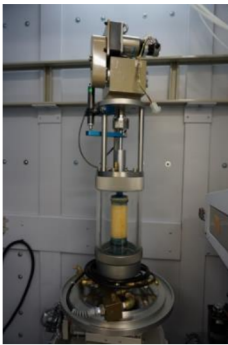
Figure 1. Whole view of the triaxial compression test apparatus. This apparatus was developed so that it can be operated inside the X-ray CT scanner.
