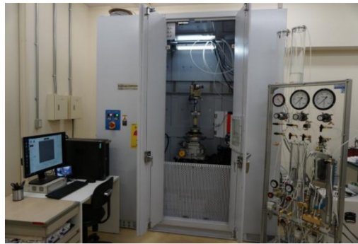
Figure 2. Whole view of the X-ray CT scanner. The maximum of X-ray tube voltage and current are 225kV and 600 \mu A, respectively. The triaxial test apparatus installed into the X-ray CT scanner can be operated from outside with the pressure and water control panel placed at the right side in the figure.
