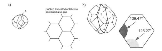
Fig. 2. Truncated octahedra as a model grain in homogenous microstructure of one-phase material: a) incorrect model plain section proposed by Ashby and Jones (1986), b) Ashby's model after correction.
