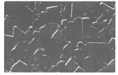
microstructure of one-phase brass, 200x
