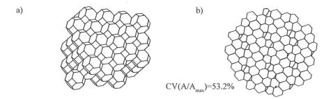
Fig. 1. Model of homogenous granular microstructure: a) agregate of grains, b) representative plane section.  $CV(A/A_{max})$  – coefficient of variation of relative plane section area.
