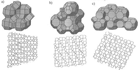
Model Williams' structures and their random plane sections: a) W1 structure, b) W2 Fig. 3. structure, c) W3 structure.
