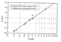
Fig. 7. Relationship between mean plane section area of grains  $E_N(A)$  and mean grain volume  $E_N(V)$ .
