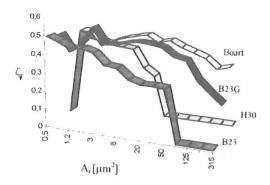
Areas occupied by cobalt binder were assessed through two distributions - of plane section area and of chord length determined with intercept method. Parameters of these distributions (Table 3) show considerable differentiation of both mean size of cobalt binder islands and their size inhomogeneity. The finest islands occurred in H30 grade, then in B23, B23G and Boart specimens. The highest inhomogeneity of cobalt binder areas was found in the fine grained hard
