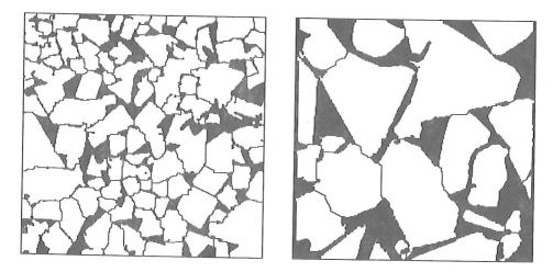
Fig. 3. Detected carbide particles (white areas) of B23 (left) and B23G (right) grades.
