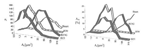
Fig. 4. Statistical (left) and geometrical (right) distributions of carbide particles size.
