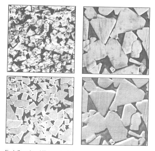
Fig. 1. Comparison of SE (top row) and BSE (bottom row) images of B23 (left) and B23G (right) grades
