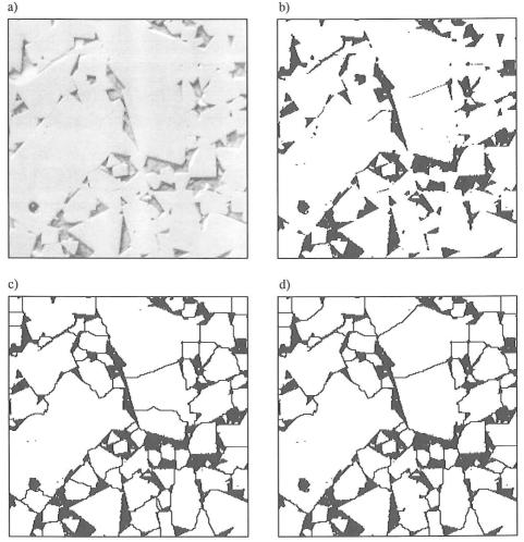
Fig. 2. Application of morphological operations in image processing (Boart specimen): initial numerical image (a), detected binary image (b), image (b) after segmentation (c), and final image of cobalt path (d).
