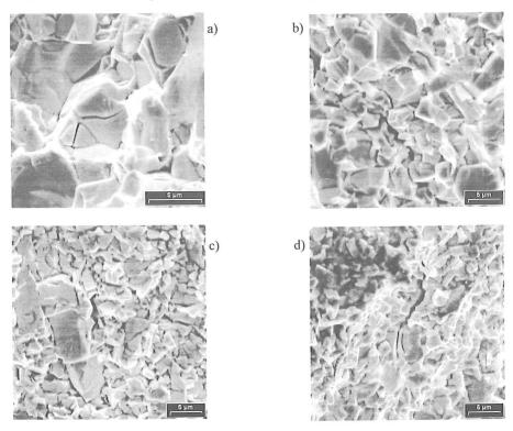
Fig. 4.SEM images of the sintered specimens subjected three points bending tests
