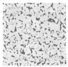
Fig. 1. Examples of the sintered carbides microstructure: B23G grade, light microscopy x2000 (left) H30 grade, SEM, BSE mode x5000 (right)
