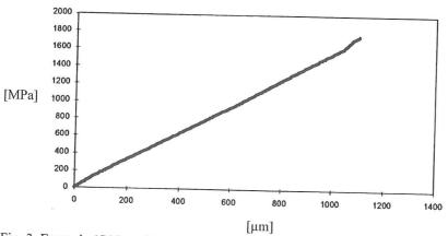
Fig. 3. Example (G10 grade) stress-deflection curve recorded during the three points bending test.
