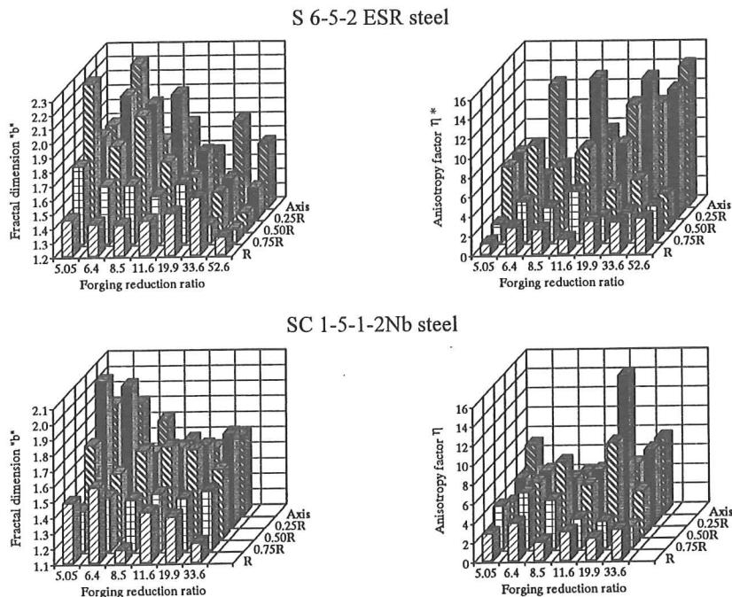
Fig. 4. Results of quantitative evaluation of carbide particles distribution inhomogeneity on transverse cross-sections of the investigated bars.
