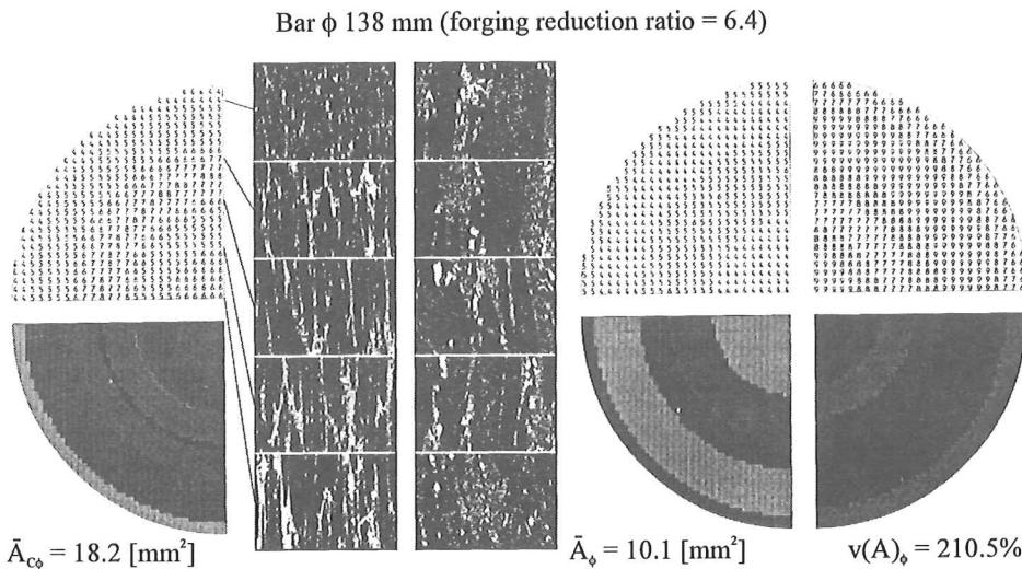
Fig. 3. "Structural maps" showing carbide clusters and particles size variation on transverse cross-section of S 6-5-2 ESR high-speed steel bar (notation as in Fig. 2).
