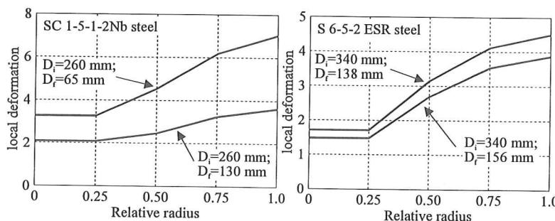
Fig. 5. Example local deformation distributions on transverse cross-section of investigated bars, determined by finite element method.
