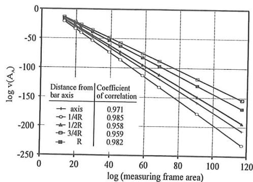
Fig. 1. Log-log plot of coefficient of variation of carbide particles area fraction, measuring frame area in systematic scanning and variance analysis method.
