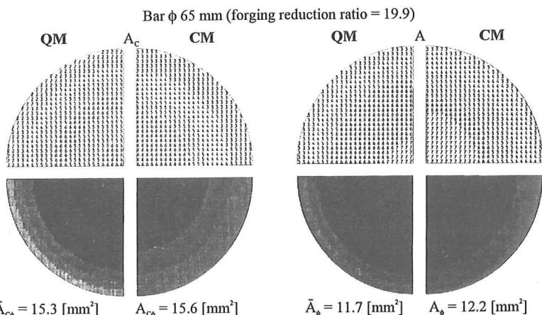
Fig. 7. Comparison of the results of quantitative evaluation (QM) and computer modelling (CM) of carbide clusters and particles size on transverse cross-section of SC 1-5-1-2Nb steel bar (notation as in Fig. 3).
