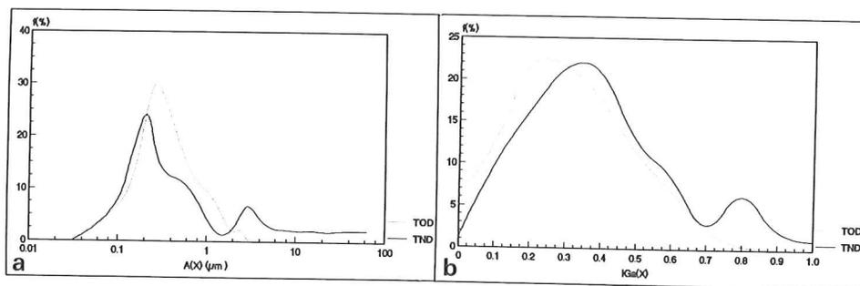
Figure 2 : Effect of the presence (TOD) or not (TND) of the phosphoric ester dispersant agent on the dispersion of  $BaTiO_3$  powder : a) granulometric distributions of projected surfaces,  $A(X)$ ; b) granulomorphic distributions of the geodesic lengthening according to the surface area,  $IG_a(X)$ .
