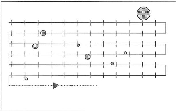
Fig.1. Modified point counting method executed with an image analysis system.
