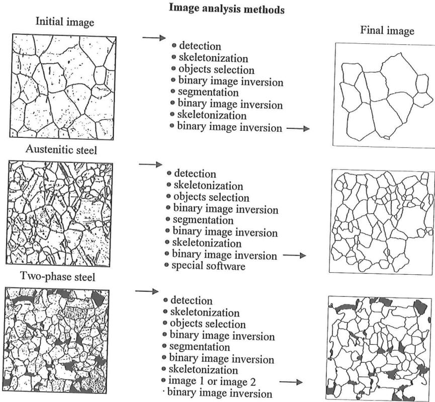
Fig. 4. Examples of image analysis methods application for an elimination of preparation artefacts and particles as well as for grain boundary reconstruction in steel granular microstructure examination.
