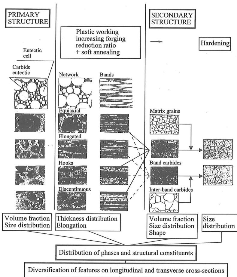
Fig. 1. Model primary structures of high speed steels and corresponding secondary structures in bars with small and large forging reduction ratio.
