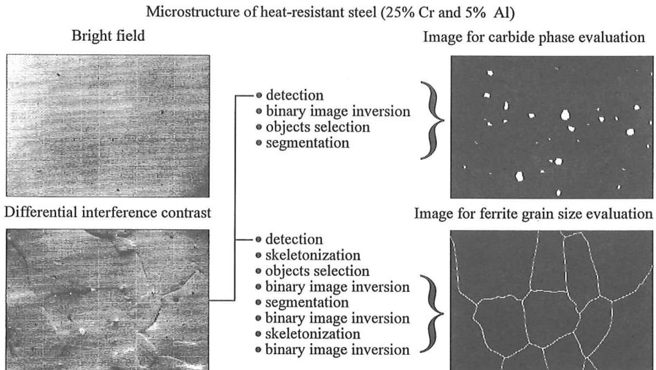
Fig. 3. Role of microscopic observation and image analysis methods in quantitative metallography of steel.
