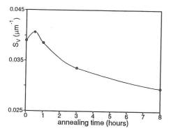
FIG.5. The dependance of  $S_V$  on the annealing time for the process of continuous recrystallization observed during annealing at 400°C
