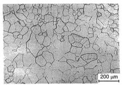
FIG.1. A microstructure characteristic of an annealed  $\alpha$ -Fe
