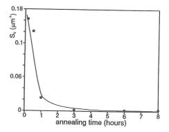
FIG.6. The dependance of  $S_V$  on the annealing time for the process of discontinuous recrystallization observed during annealing at 500°C
