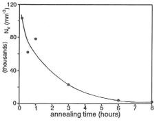
FIG.7. The dependance of  $N_V$  on the annealing time for the process of discontinuous recrystallization observed during annealing at 500°C
