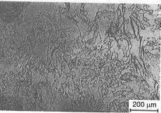
FIG.4. Image of grain boundary network of the material after extrusion and the annealing at 500°C for 0.5 hour
