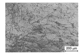
FIG.2. Grain boundary network revealed on a longitudinal section of  $\alpha$ -Fe after 50% reduction in compression
