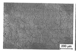
FIG.3. Image of the grain boundary network of the material after extrusion and the annealing at 400°C for 0.5 hour
