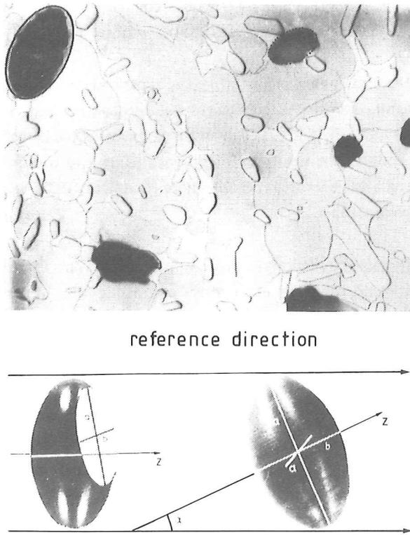
Fig. 1: Determination of axial ratios of sectional ellipses
