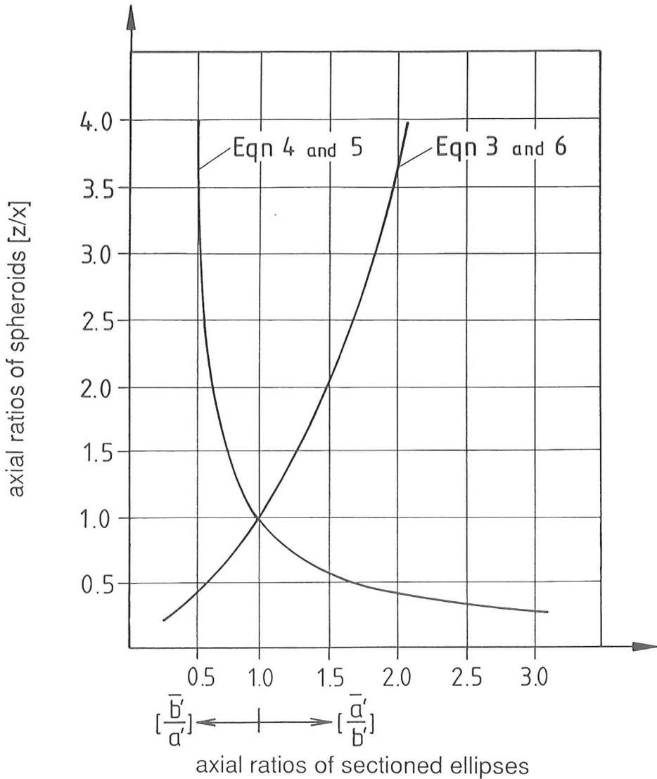
**Fig. 2:** "Spatial " axial ratio of spheroids as a function of "plane" axial ratio of sectioned ellipses
