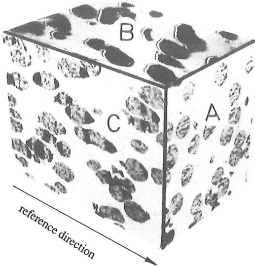
Fig. 3: Sections through a two phase material in order to determine the orientation factor
