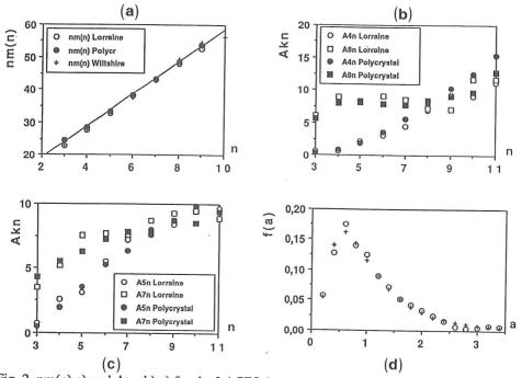
Fig. 2. nm(n) a) and  $A_{kn}$  b) c) for the LACES (open circles and squares) and for a planar cut of an alumina polycrystal (full circles and squares), nm(n) for the Wiltshire (crosses) is also shown in a). d) Distribution of the reduced areas a=A/<A>\* of the LACES : observed (open circles) and calculated (crosses, Eq.4).
