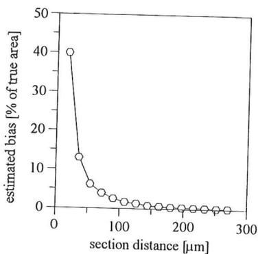
Fig. 4. Estimated bias of surface area estimation, in % of true area.
