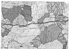
Fig. 3c. Dolomite after tensile test. x 100.
