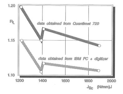
Fig.1. Profile line parameters versus work of fracture
