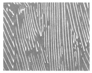
Fig. 2. Coarse pearlite. SEM, x2500, etched by picral.
