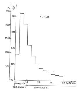
The empirical distribution of the random distribution reciprocal was presented in Table 3 and Fig.5. In the range from  $1.25\cdot10^3$  to  $2.5\cdot10^3$  mm<sup>-1</sup> the distribution function in Fig.5 is drawn with the broken line – accuracy of single  $l_{\rm r}$  measurements disabled of more precise estimation of the distribution in this range.
