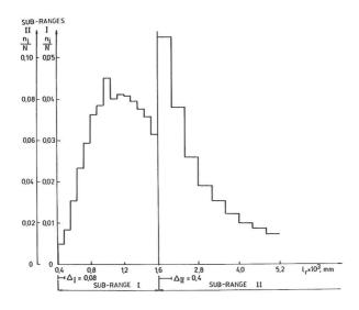
Fig. 6. Empirical distribution of random spacing. Sub-range I - SEM ,sub-range II - optical microscope.  $\triangle_{\rm I}$  ,  $\triangle_{\rm II}$  - class interval width in sub-range I and II, respectively.
