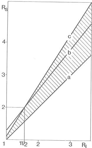
Fig.2. The RL-RS space with theoretical bounds: a - lower bound, b and c - upper bounds according to Underwood and Wojnar.
