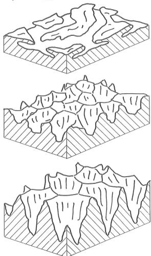
Fig. 3. Model fracture surfaces. From top to bottom: relatively flat, randomly curved, deep.
