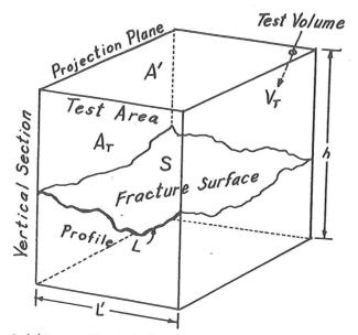
Figure 1. Arbitrary Test Volume Enclosing a Fracture Surface.
