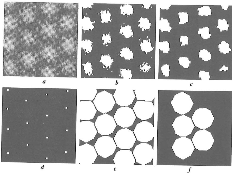
Fig. 2. Illustration of the sequence for building a template image, on a small 100X100 pixels image. a. initial image; b. thresholded image; c. after opening and closing by a 3X3 square; d. geodesic centers (dilated to be seen on the figure); e. thickened image, mask areas; f. final template image after border removing
