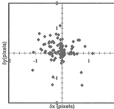
Fig. 4. Scattering diagram showing the difference  $\delta y$  in y coordinate vs. the difference  $\delta x$  in x for each point, measured using 2 template images obtained from two different thresholds. Most of the 136 points are packed in the center zone of the diagram.
