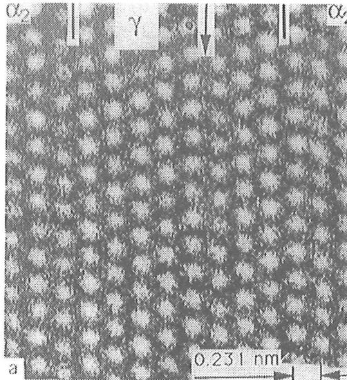
Fig. 1. HRTEM image of a Ti-30%Al alloy showing alternated  $\alpha_2$  and  $\gamma$  layers (courtesy R. Bonnet and M. Loubradou). The image is 505X554 pixels, with  $6 \cdot 10^{-3}$  nm/pixel.
