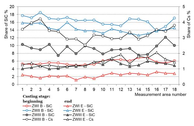
Figure 5. Percent content of the reinforcing particles of SiC and Cs in the examined ZWI, ZWII and ZWIII pistons
