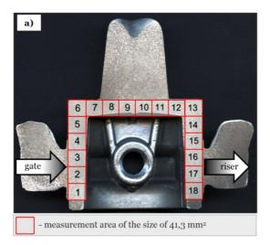
Figure 2. Cross-section of the cast piston with marked locations where the content of reinforcing particles was examined
