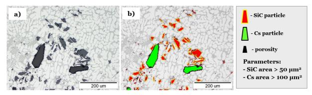
Figure 4. Example of microstructure obtained in ZWIII piston (a) with marked particles of SiC and Cs (b)  $\,$
