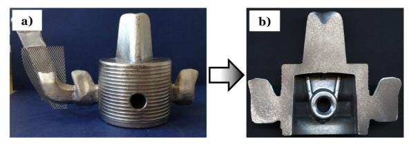
Figure 1. Cast piston (a) and its cross-section (b)
