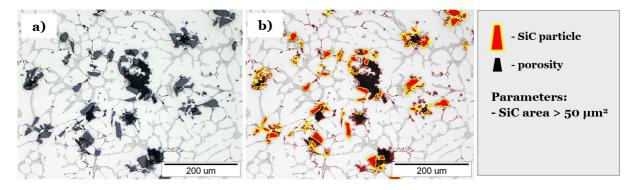
Figure 3. Example of microstructure obtained in ZWI piston (a) with marked SiC particles (b)
