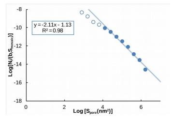
Figure 2. Graph showing power law distribution of porosity measured on SE-Image shown in Figure 1 and normalized by the measured image area. Segmentation is assumed to be valid for pores larger than 9 pixels which corresponds to  $\sim 10^4$  nm<sup>2</sup> at the given image resolution.
