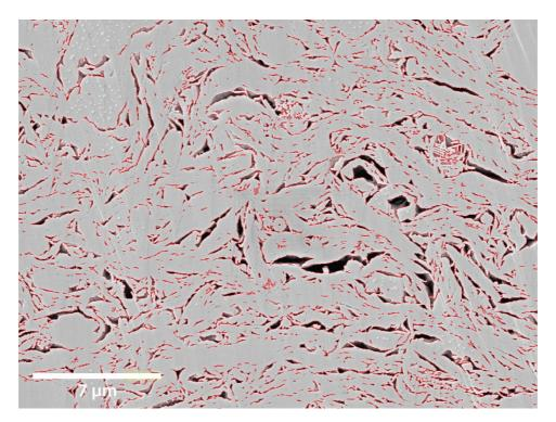
Figure 1. Secondary Electron mage showing porosity in clay. Over 5000 pores were segmented (red outline) in this field of view. The measured porosity is 11.95%
