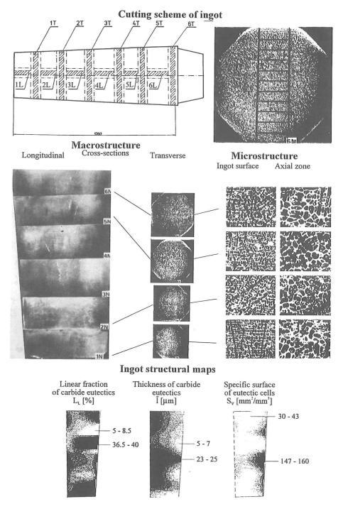
Fig. 2. Macro- and microstructure of SC 12-0-5 high-speed steel ingot (375/285x1080 mm - 900 kg).
