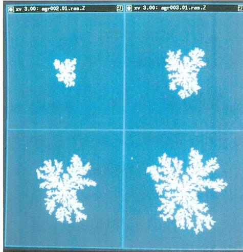
Fig.1. Generation of a random aggregate by rule A: 500, 1000, 1500 and 2000 iterations.
