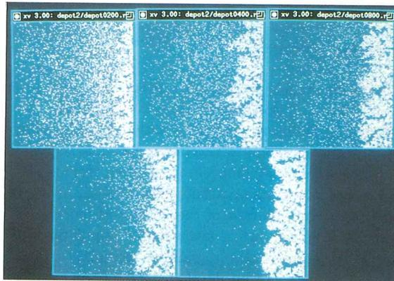
Fig. 6. Deposition and packing of aggregates (rule B after 200, 400, 800, 1600, and 3200 iterations)
