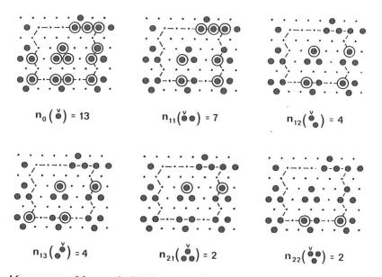
Fig. 1 : Measurement of the specific E.P.C. on a  $8 \times 8$  binary image. The symbol « v » designates the origin of the configuration and each configuration is taken into account only if its origin belongs to the field of measurement (dotted line). The origin is then located by a circle.
