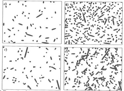
Fig.2. Plane section of computer simulated SSI model X (a: p=0.05; b: p=0.2) and Boolean model with the same volume content and grain size(c: p=0.05; d: p=0.2).
