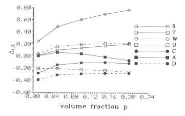
Fig.5. Relative differences  $\Delta_{k,z} = (\mu'_{k,z} - \mu'_{k,x})/\mu'_{k,x}$  for selected models.
