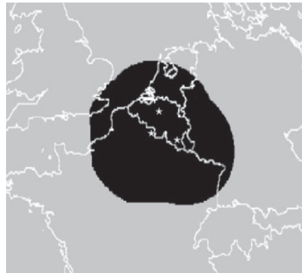
Figure 1. Location of the three radars (Zaventem, Wideumont and Avesnois) used in composite images and corresponding 240 kilometers useful radius.
