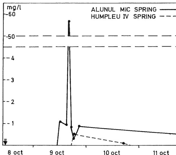
Figure 2 : Moment of injection of 1 kg uranine - October 8, 15.00 p.m., Ponorului valley stream sink
