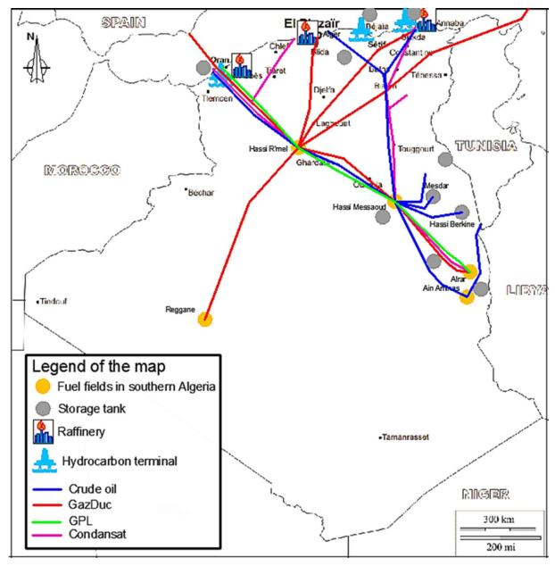
**Figure 2.** Approximate map of extraction veins and pipeline transport of fuel energy in southern Algeria to refineries and oil ports in northern Algeria. Source: The authors, 2022, are based on data from the hydrocarbon pipeline network description document provided by sonatrach in 2021 - https://sonatrach.com/wp-content/uploads/2021/02/DESCRIP-TION-DU-RESEAU-DE-TRANSPORT-PAR-CANALISATION-DES-HYDROCARBURES-TARIF-DE-TRANSPORT-ANNEE-2021.pdf
