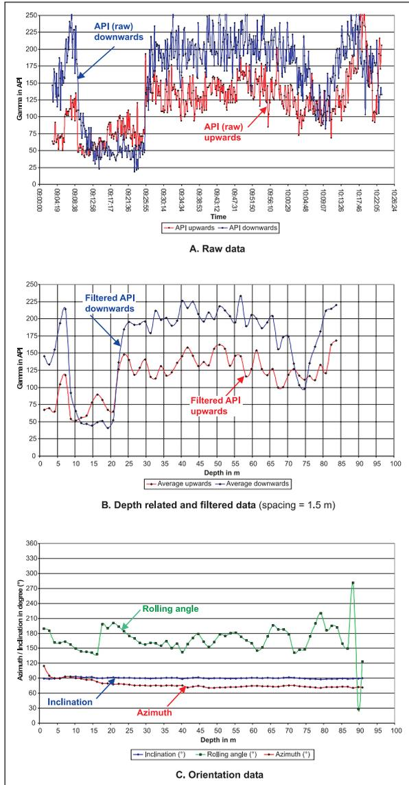
Figure 5. Typical measuring curves: A. Raw data B. Depth related and filtered data C. Orientation data.
