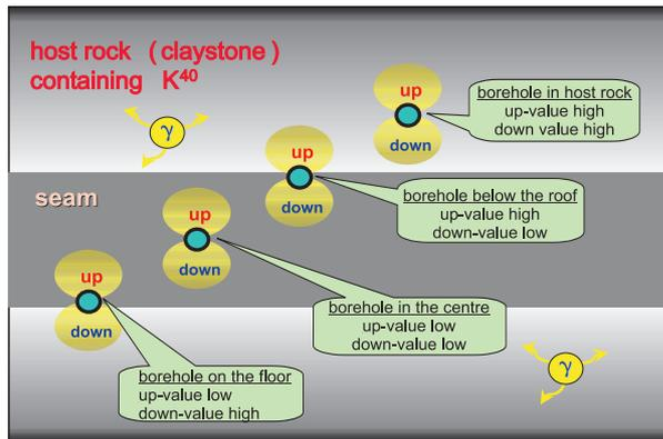
**Figure 2.** Section through Directional Gamma-Shuttle in different positions relative to the seam.
