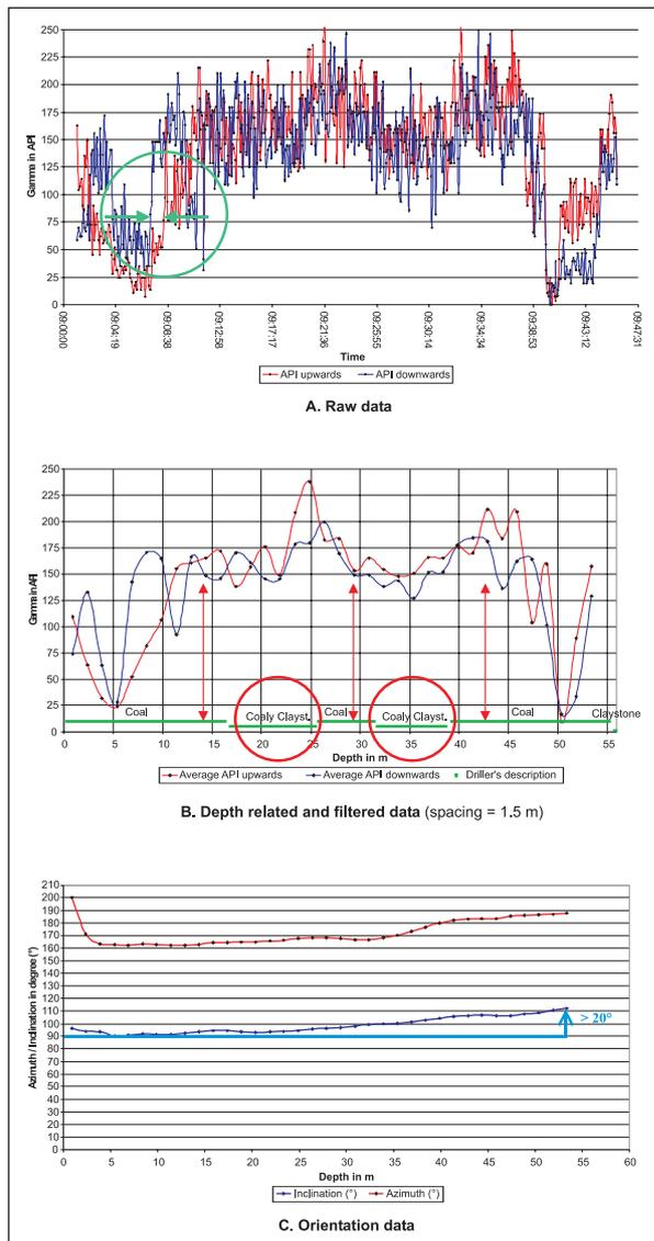
Figure 7. 1<sup>st</sup> measurement: A. Raw data B. Depth related and filtered data C. Orientation data.
