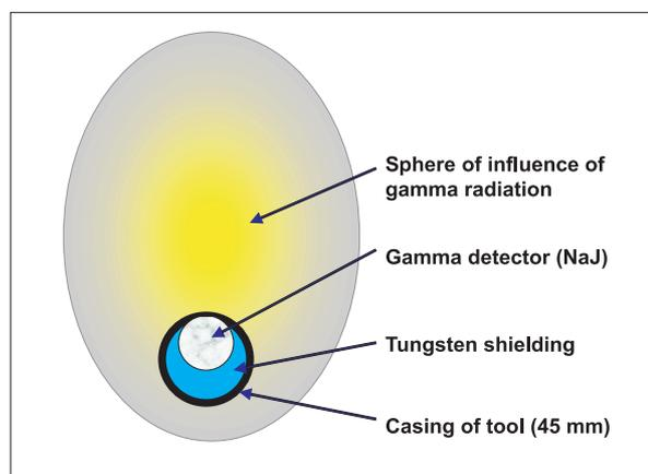
Figure 1. Section through directional gamma detector.
