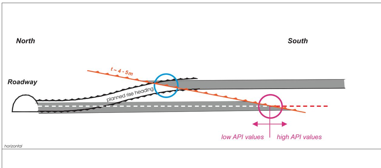
Figure 6. Cross-section posing the problem prior to drilling and logging.
