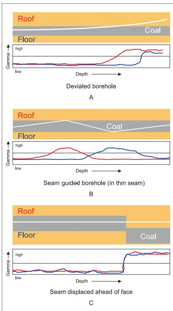
**Figure 3.** Exemplary situations and measuring curves: A. Deviated borehole B. Seam-guided borehole C. Seam displaced ahead of face.
