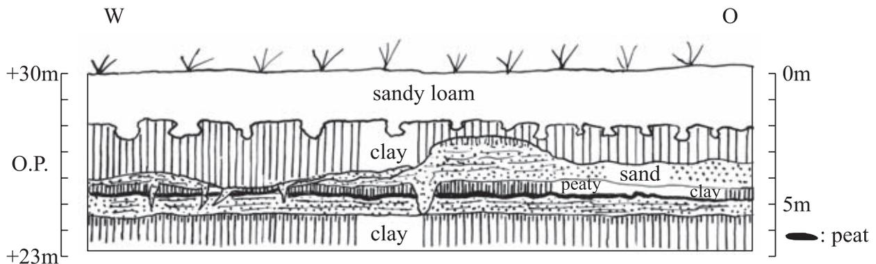
Figure 11. Section of the clay pit 12, exposed at Beerse in 1959.
