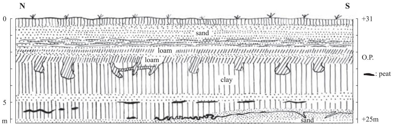
Figure 8. Section of the clay pit 7, visible in 1959, at Beerse.
