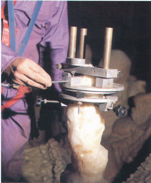
Figure 5. Grotta del Cervo cave: the azimuth of the principal dislocations in the growing axis of a stalagmite is measured by using a specific instrument (Fig. 6).
