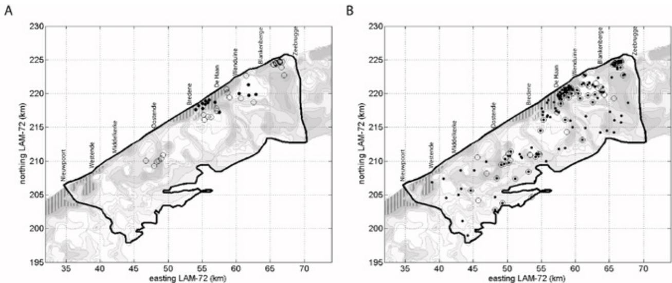
**Figure 5.** Comparison between the new data and the 1974 map in case of borehole logs (A) and water quality data (B). (•) indicates where the observation corresponds with the 1974 map, (o) where the new data do not confirm the map information.
