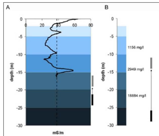
**Figure 4.** Illustration of the update procedure in case of a borehole measurement (A) and water quality data (B). The intervals according to the original map are indicated as well the classification in the old interval (black bar) and the reclassification (grey bar). The dotted line (A) gives the threshold value of 37.5 mS/m.
