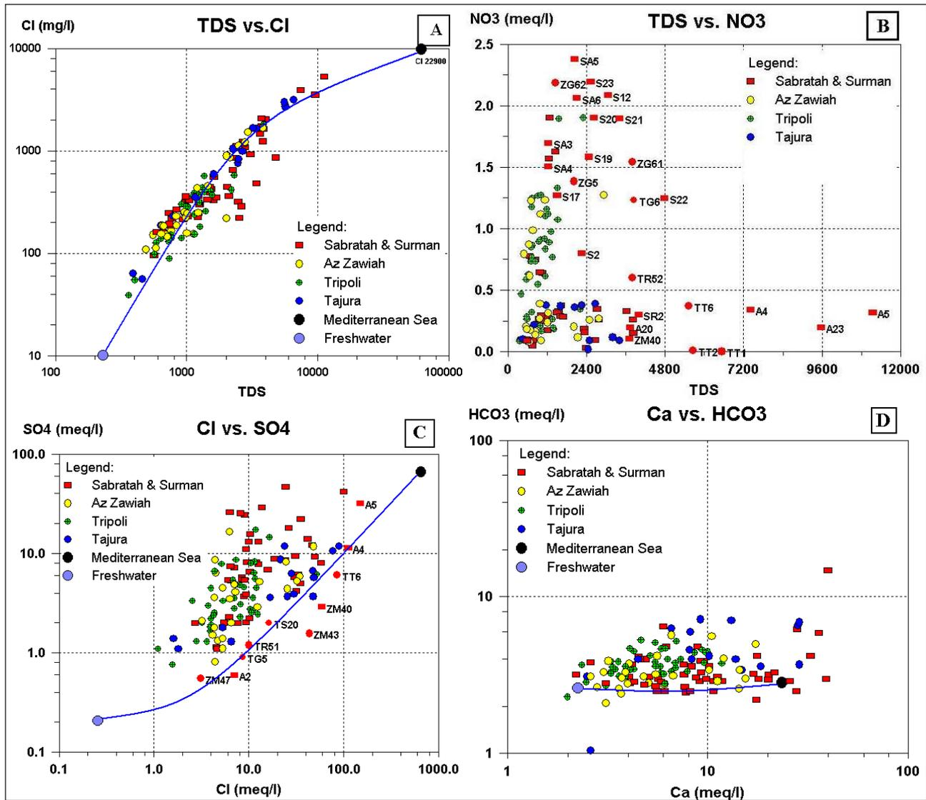
**Figure 5A-D.** TDS vs. Cl<sup>-</sup>, TDS vs. NO<sub>3</sub><sup>-</sup>, Cl<sup>-</sup> vs. SO<sub>4</sub><sup>2-</sup> and Ca<sup>2+</sup> vs. HCO<sub>3</sub><sup>-</sup>. The curves represent mixing of freshwater and Mediterranean Seawater.
