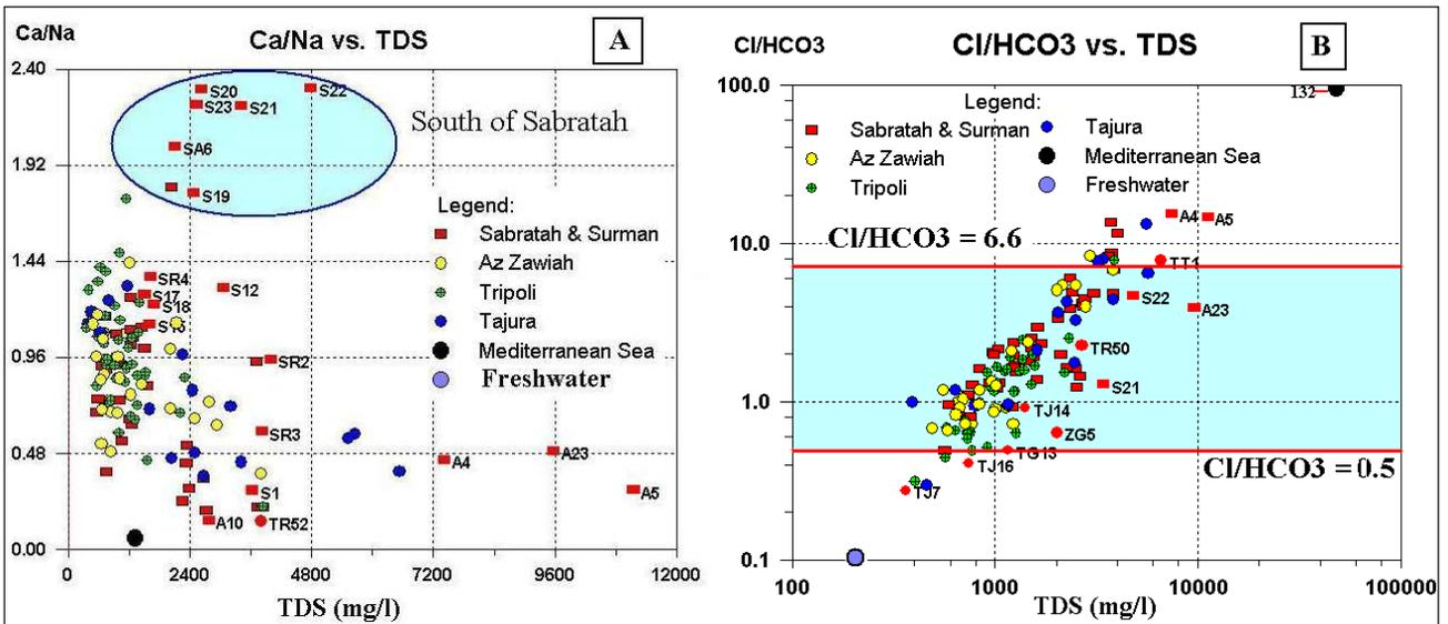
Figure 10A-B. Ionic ratios Ca/Na vs. TDS and Cl/HCO<sub>3</sub> vs. TDS.
