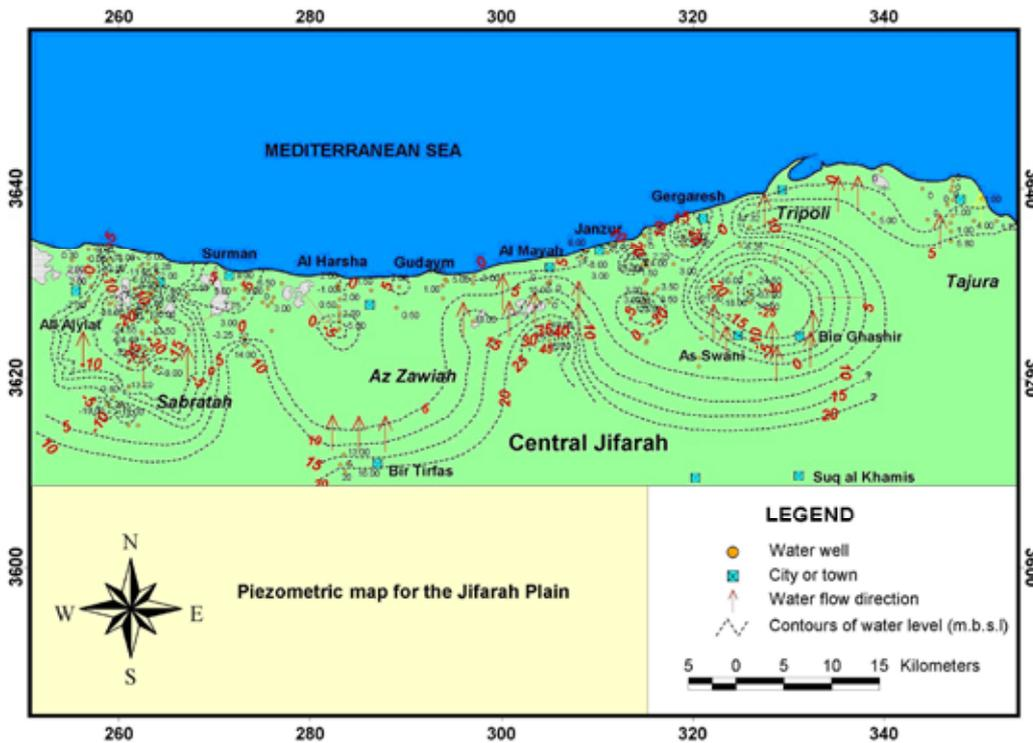
Figure 4. Piezometric map for the coastal area of central Jifarah.
