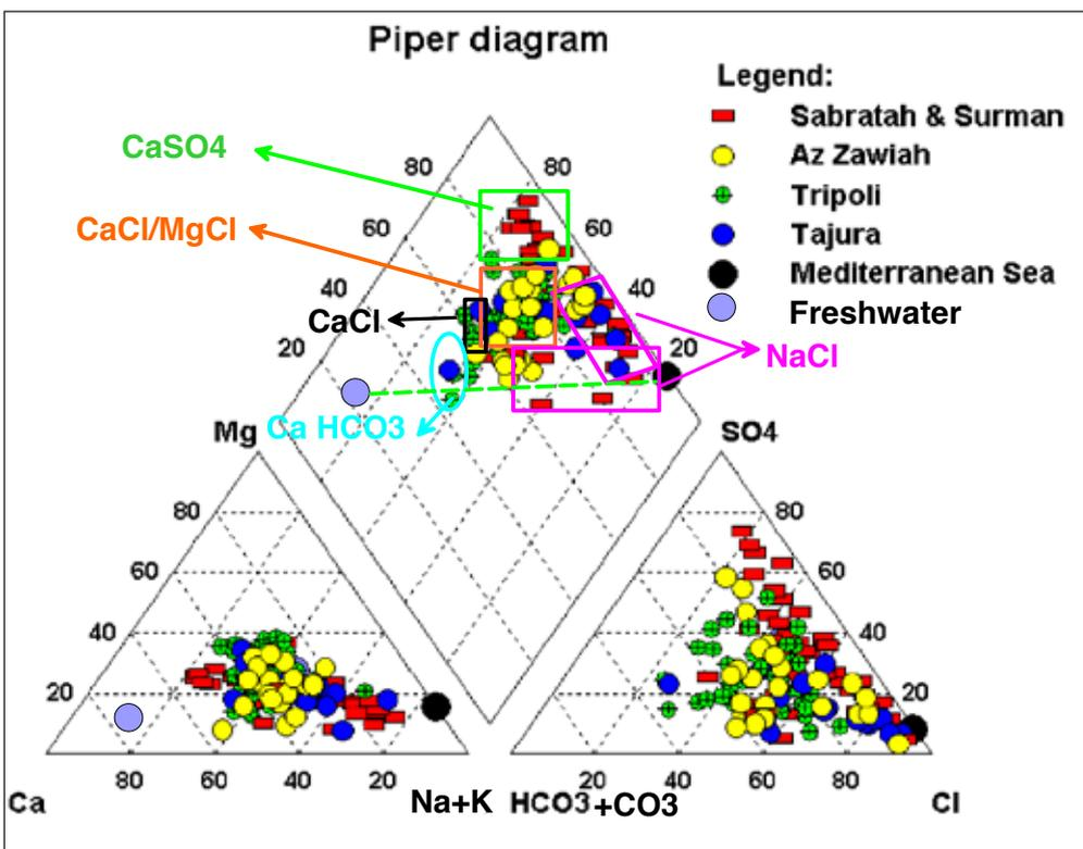
Figure 11. Water types according to Piper diagram.
