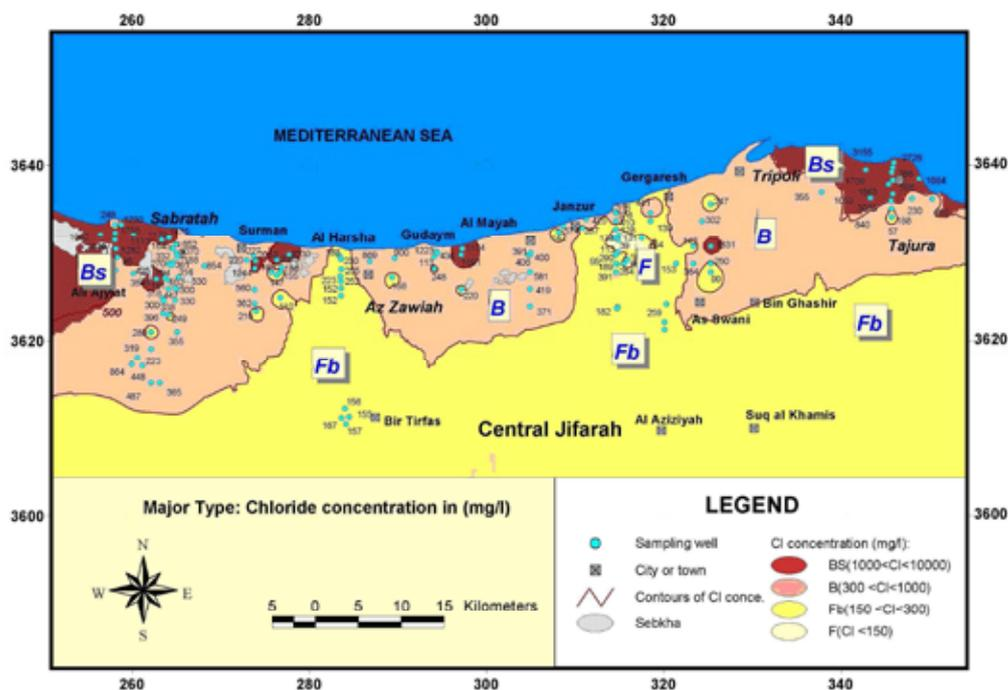
Figure 12. Main water type (chloride concentration).
