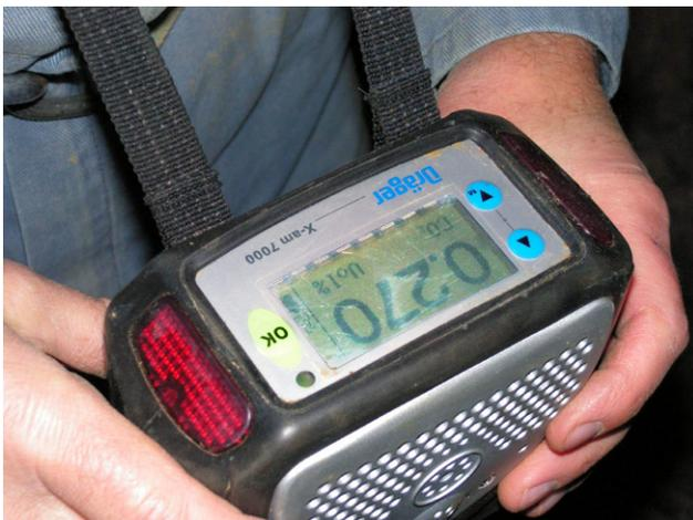
Figure 3. X-am 7000 by Draeger, infrared portable gas analyzer. Used in our current surveys since 2008.
