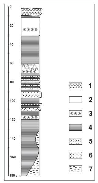
**Figure 8**. Lithostratigraphic column of the "Petites Fontaines" sedimentary profile in the Han-sur-Lesse cave (in insert, Fig. 7). 1. Speleothem. 2. Non laminated clay. 3. Redox front. 4. Brown non laminated clay. 5. Silt. 6. Thin sand. 7. Grey laminated clay.
